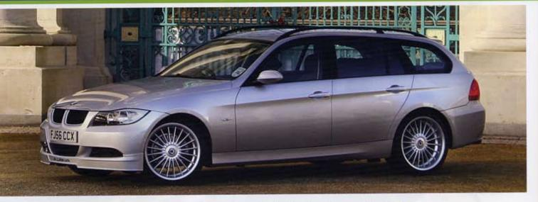
has increased power but class leading performance too.0-60 is achieved in 7.5secs with a top speed of 143mph with max torque of 302 lb-ft (410 Nm) at 2000rpm compared to the 320d at 8.5 sec, 136mph and 251 lb-ft (340 Nm)
